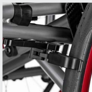
Innovative, "Light" brakes made of aluminium and swivel-mounted
