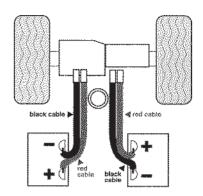
Your scooter comes supplied with two battery cables. Attach the red wire of the first cable to the (+) terminal of the first battery. Attach the black wire of the first cable to the (-) terminal of the first battery. Repeat this procedure for the second battery.
