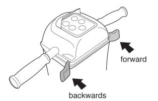
**Forward/Reverse:** Push the right lever to move forward, push the left lever to move backwards.
